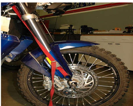
It's critical to tie the forks up to the rafters, as when the triple clamp is off, the forks can roll away from the bike.
