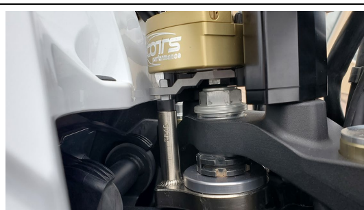
Finished kit with linkarm and tower pin properly aligned.
