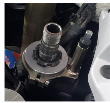
Install the first castle nut to the tension it was before coming off. This nut adjusts the tension on the head bearing. See factory specs.
