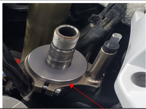
Install the newly supplied bearing shroud and be sure it's not touching the frame bracket
