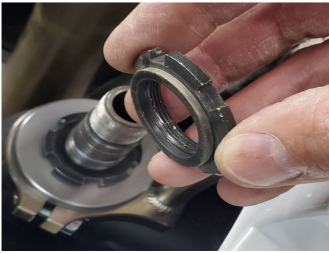
Install the second castle nut and washer in between, this is the lock nut, or jam nut.
