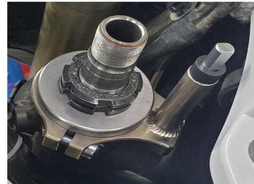
Tighten nut #2 against the first nut and align the castle nuts so the slots match allowing the tab to drop into the slots.
