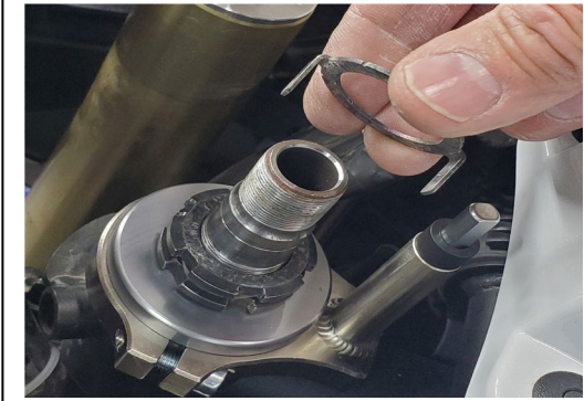
Install the tab so it fills both sets of slots on the castle nuts
