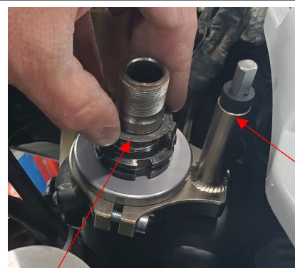
Tab being installed into aligned slots on both castle nuts.
