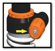
4) Electrical Preload Adjuster Push the button from the Tractive control panel. Push "Hard" to increase the preload and push "Soft" to decrease it. (See picture)
