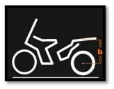
Put the vehicle back on the wheels. (without rider) and repeat the measuring procedure.
