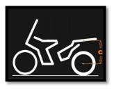
d) Then take the same measurements with the rider and equipment on the motorcycle. It is important that the rider is balancing on the correct riding posture and repeat the measuring procedure one more time.
