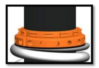
3) Hydraulic Preload Adjuster Turn the Hydraulic Adjuster knob to set the preload. Turn clockwise to increase the preload, turn counter clockwise to decrease it. (See picture)
