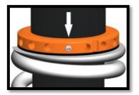
2) Mechanical Preload Adjuster with contra nut.
