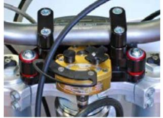
approximately 11 mm to 25 mm, depending on the bike. Lower bend bars are available from Scotts upon request. SUB mounts are designed for oversize bars. Reducer bushings are available to use Standard bars. Each kit comes complete with all necessary hardware for mounting. Rubber Mounted submounts are available for KTM, Husky, Husaberg, Beta and Yamaha.
