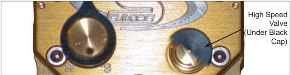
We have pre-set the High Speed Valve to One Turn Out from the Full Stiff Position before shipping. Before changing this, ride with the stabilizer for some time to get the feel of it. Then, adjust in 1/8th turn increments, until you find a setting you like.
