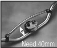
This illustration shows the required 40 mm of clearance between the main bar and the crossbar for mounting a SCOTT'S Seering Stabilizer.
