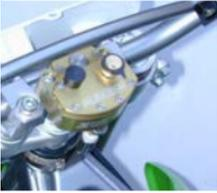
Some applications require the Stabilizer to be mounted in the “Reverse” position in order to clear crossbars, computers, or other items. This position can be achieved by reversing the stepped link arm. A link arm puller (Scotts Part Number 9007-03) is recommended for this operation. (Flat link arms cannot be reversed.) Reversed mounting does not effect the bracketry or function of the stabilizer. It is simply an option to accomodate mounting differences.
