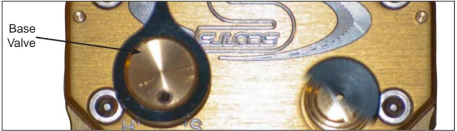
The Base Valve adjusts the amount of resistance you feel as you turn the bars left to right.. As you turn this knob clockwise (to the Right) you will increase the "stiffness" of the stabilizer. Counter clockwise would be less stiff, a softer feeling.
